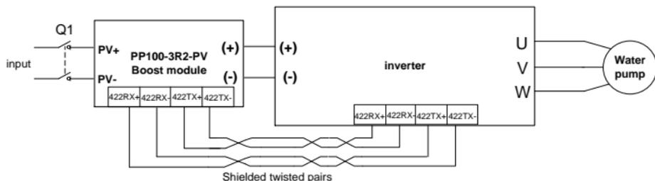
Fig A.1 Connection between the boost module and inverter
