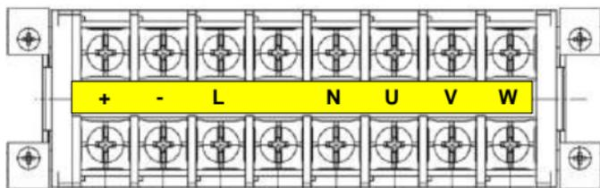
Fig C.6 Wiring terminals of S2T/SS2T models for inverters  $\leq 2.2\text{kW}$
