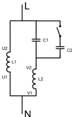
Internal wiring of the single-phase motor winding after removing the starting and running capacitor:
