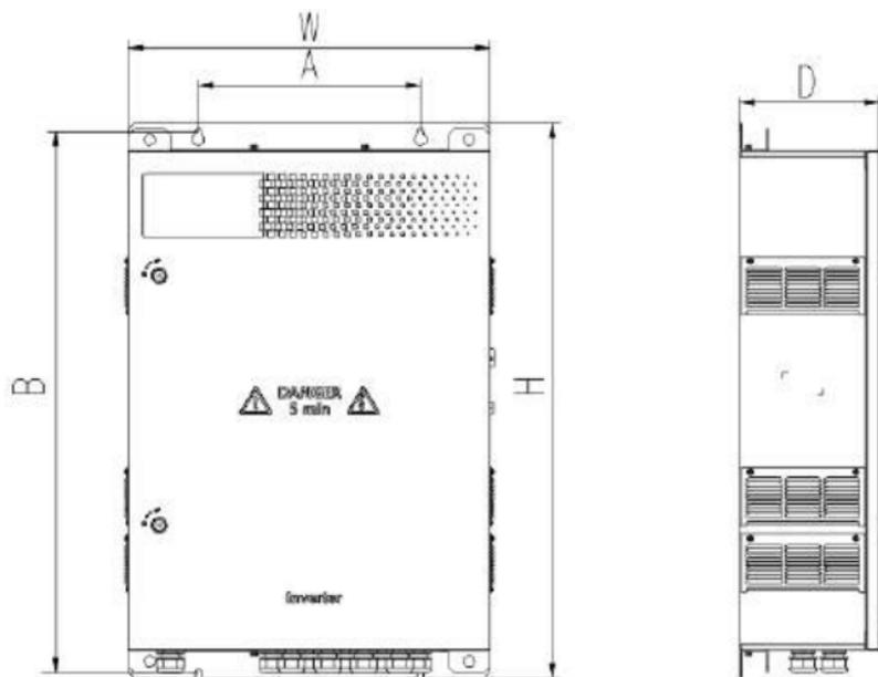
Fig C.3 IP54 inverter dimensional drawing
