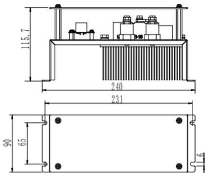
Fig C.2 Switching module installation dimensions (unit: mm)
